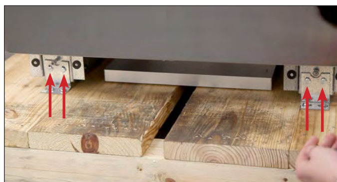
FIG. 7. Shipping bracket bolt locations.
