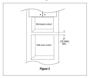
• The floor of the opening should be constructed of plywood strong enough to support the weight of the oven and floor load (about 100 pounds/45 kg). The floor should be level and 90° with the face of the cabinet for proper installation and operation of the oven. Be sure to check the local building code as it may require that the opening be enclosed with sides, ceiling and rear partition. The proper functioning of the oven does not require the enclosure.
