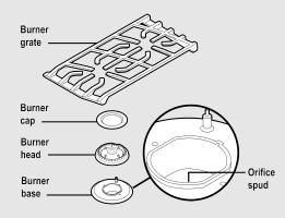
2. Using a 9/32" or 7 mm nut driver remove the top burner orifices. These may be accessed through the opening in the burner base
