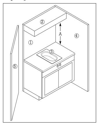
**The minimum spaces** that must be maintained between the appliance cooking surface and the horizontal surface above the cooking top shall be:
