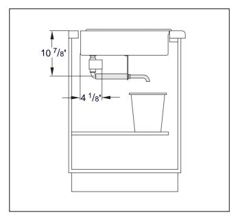
If no drain connection is available, the **drain installation set (AG 060-000)** allows you to drain the cooking liquid into a suitable receptacle (e.g. a 10 l bucket).
