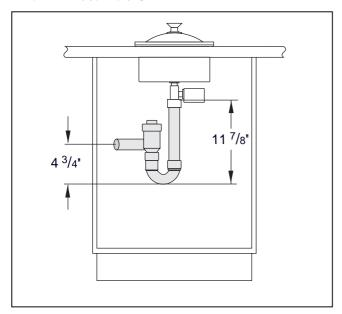
A permanent drain connection using our **drain installation set (AG 050-000)** is recommended. This requires a drain connection in the base cabinet. A non-return valve must be installed. It can be connected permanently or with a free fall.
