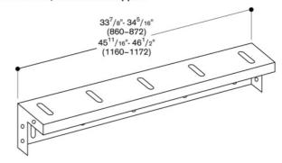
AL400790 Retractable downdraft with LED lighting Stainless Steel Width 36 inches Comes without blower Air extraction/recirculation with AR 400/401 blowers or AR 413
