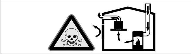
Room air-dependent heat-producing appliances (e.g. gas, oil, wood or coal-operated heaters, continuous flow heaters or water heaters) obtain combustion air from the room in which they are installed and discharge the exhaust gases into the open through an exhaust gas system (e.g. a chimney).
