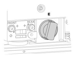
(6) Ensure the filter is in the locked position (E). Remove filter removal tool and close the freezer drawer.
