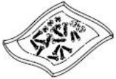
Parts Bag (includes 4 flat head screws #10-2", 8 screws #8-3/4", 4 Nuts #10-32, 2 Wall anchors and 2 Washers 3/16" ID x 3/4" OD)
