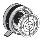
4. Insert the filter behind the bottom tab and snap it into place at the top.
