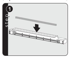
Apply adhesive tape to grille assembly. Trim excess
