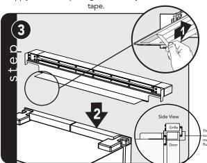
Remove adhesive backing. Align and position grille on top of unit so that the face of the grille and the face of the door are flush. Firmly press the grille assembly down so the adhesive adheres to the cabinet.
