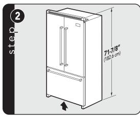
Raise the unit up until the measurement from the floor to the top of the grille assembly is 71-7/8 inches.
