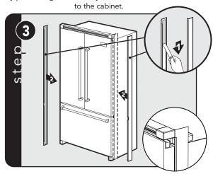
Shim trim has adhesive backing on both sides. Remove adhesive backing on refrigerator side only. Fit the shim trim to the front of the unit first. With center hinge, the shim trim will have a cutout. Use the cutout to locate the height of the shim trim.
