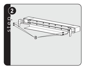
Attach spacers, included in the kit, to the grille assembly with four screws.
