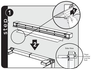
Apply tape to grille assembly. Do not attach spacers. Remove adhesive backing. Align and position grille on top of unit so that the face of the grille and the face of the door are flush. Firmly press the grille assembly down so the adhesive adheres
