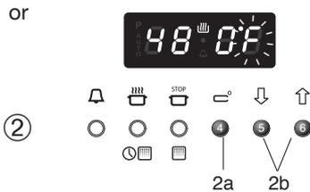
**Note:** When °F or °C becomes steady the value shown on the display indicates the oven cavity temperature until set temperature is reached. If set temperature is less than inside oven temperature, the display shows the set temperature.
