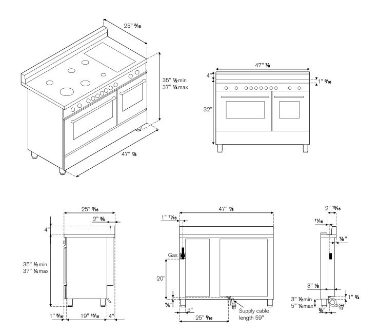
Bertazzoni recommends to operate the appliance after it has been installed in a cabinet. The kitchen cabinets shall be made of materials capable of withstanding temperatures at least 117°F (65°C) above room temperature in order to avoid possible damage to the cabinets during oven usage. For further installation instructions refer to the installation manual.
