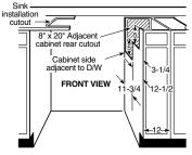
Cabinet cutouts for offset single and double bowl sinks. Dishwasher not provided with complete enclosure. Enclosures for sides, top, bottom, and back must be provided by installer at time
