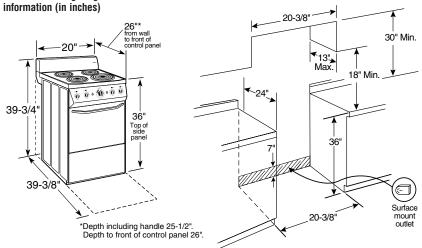
**Note:** Compact 20" Electric Ranges conform to U.L. requirements for 0" spacing from range to adjacent walls below countertop.
