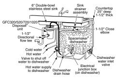
A close-fitting elbow or special shallow sink strainer is necessary to provide clearance between sink drain and dishwasher. Dishwasher furnished with 1/2" I.D. drain hose, 78" long. If using copper tubing, 2" length of 1/2" I.D. rubber hose must be provided to connect copper tubing to pump outlet. Disposer should have 7/8" I.D. dishwasher drain connector.
