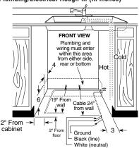
Plumbing: Hot Water Only: Use 3/8" O.D. copper tubing or 1/2" O.D. plastic tubing min. inlet line. Water valve has 3/8" internal threads. Hand cut-off valve is recommended.
