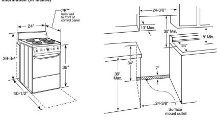
**Note:** 24" Ranges conform to U.L. requirements for 0" spacing from range to adjacent walls below countertop.
