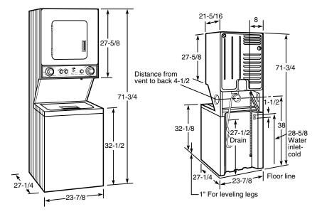
**WSM2480D: Gas dryer**—This appliance should be connected to an individual, properly-grounded branch circuit with a three-prong grounding-type receptacle and 120-volt single-phase 60 Hz electrical service and should be protected by 15 or 20-amp time-delay fuses or circuit breakers. This appliance is equipped with a 6-foot long flexible U.L. listed 20-amp power cord to match a 15-amp receptacle.
