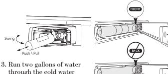
through the cold water dispenser (about 5 minutes) to remove air from the system. A newly installed filter cartridge will cause water to spurt from the dispenser. Use a large pitcher or sports bottle to establish the dispenser.
