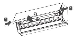
Figure 15: Detaching Filter from Indoor Unit
