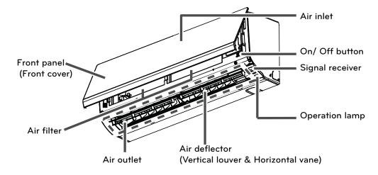
Figure 1: Art Cool Mirror Indoor Unit Basic Components
