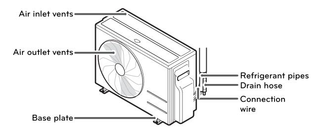
Figure 2: Art Cool Mirror Outdoor Unit Basic Components
