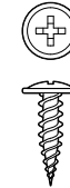
#8 x 16 mushroom washer screw (35) (12) for Side trim attachment: Fixed screw method only)
