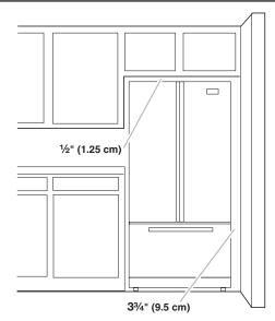
To ensure proper ventilation for your refrigerator, allow for a ½" (1.25 cm) space on each side and at the top. Allow for 1" (2.54 cm) of space behind the refrigerator. If your refrigerator has an ice maker, make sure you leave some extra space at the back for the water line connections.
