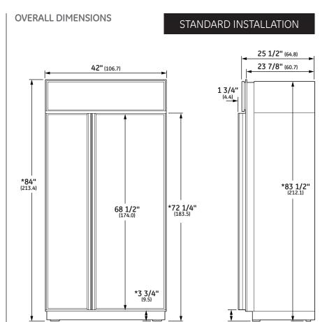
**FRONT VIEW**\* Shipping height. Use leveling legs and wheels for maximum 1" height adjustment from shipping height.
