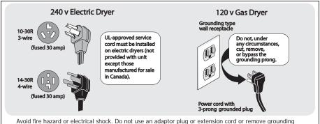
Avoid fire hazard or electrical shock. Do not use an adaptor plug or extension cord or remove grounding prong from electrical power cord. Failure to follow this warning can cause serious injury, fire or death.
