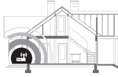
Unsuitable router position
