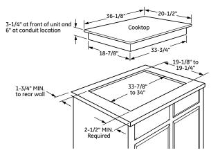
To insure accuracy, it is best to make a template when cutting the opening in the counter
