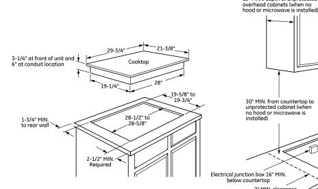
To insure accuracy, it is best to make a template when cutting the opening in the counter
