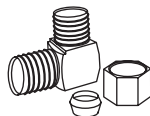
Ferrule, compression nut and 90° elbow with \frac{3}{8} " N.P.T. external threads on one end. (The other end must fit your water supply line).
