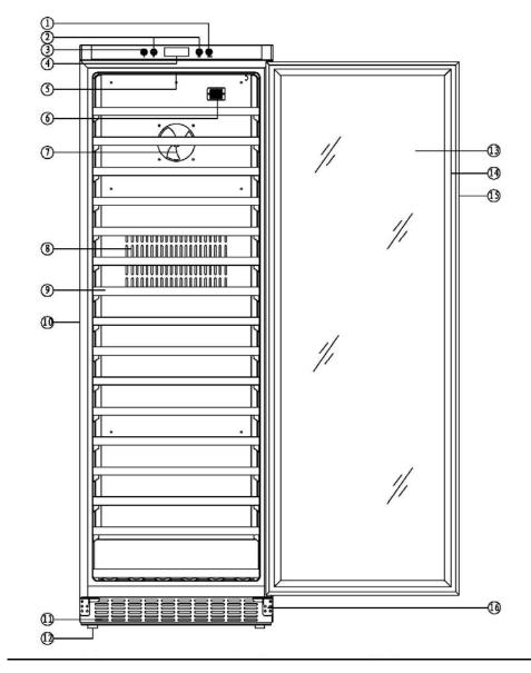
1. Light switch 9. Shelf 2. Temperature setting 10. Body 3. C/F switch 11. Exhaust window 4. Temperature display 12. Foot 5. Light 13. Glass 6. Temperature probe 14. Door seal 15. Handle 7. Fan 8. Exhaust window 16. Lower hinge Plastic humidifier tray Not shown: Compressor (rear of unit)
