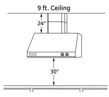
**9 ft. ceilings:** When the hood is installed 30" above the cooking surface, order two 12" duct cover accessories.
