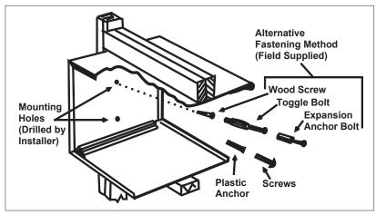
Wall Sleeve must extend a minimum of  $\frac{1}{4}$ " beyond outside wall to allow for proper caulking.
