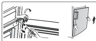
7. Place the lower door on a smooth surface with its panel upwards. Change the handle to the right side according to step 5. Loose screws⑦, detach part⑥and part⑤. Turn part⑤by 180°and then install part⑤and part⑥to corresponding position on left side together with screws⑦.
