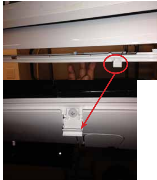
Figure 58: Remove Screws from Bottom Panel
