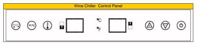
You can select temperature display setting from Fahrenheit to Celsius degree by pushing the °F/°C button/mark. Fahrenheit or Celsius degrees indicator will appear in green color in the temperature display window.
