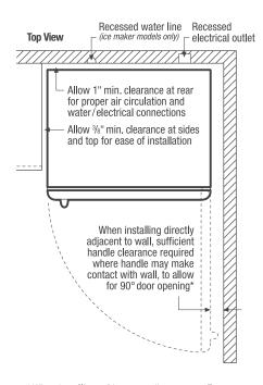
\* When installing refrigerator adjacent to wall, cabinet or other appliance that extends beyond front edge of unit, 20" minimum clearance recommended to allow for optimum 140° door swing, providing complete crisper access and removal. (Absolute 3" minimum clearance will ONLY allow for 90° door swing which will provide limited crisper access with restricted removal.)
