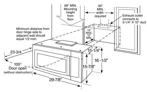
**Important Information:** When installing the microwave oven over a range, allow minimum of 2" from bottom of microwave oven to top of range backguard to allow for removal of light covers.
