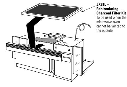
**Ventilation Options:** The microwave oven is designed for adaptation for the following three types of ventilation:
