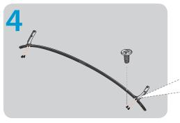
Insert 2 screws through the base into each leg as shown, and then secure the legs to the base with a screwdriver.
