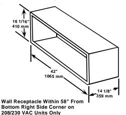
Figure 1 - Wall Sleeve Dimensions
