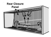
Figure 8 - Rear Enclosure Panel
