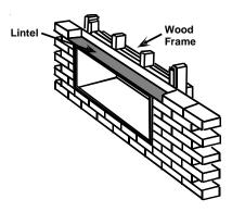
Figure 5 - Framing with Lintel
