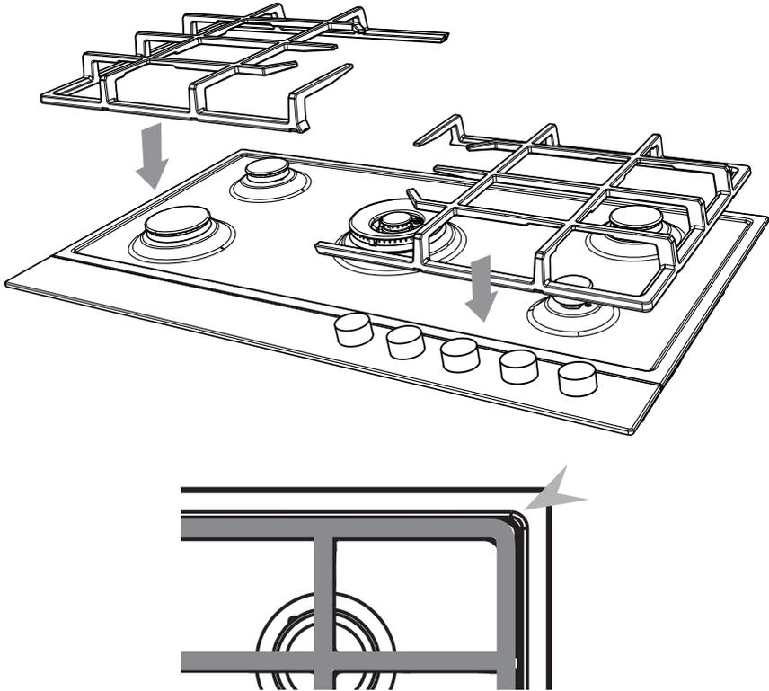
Fig.19 Correct positioning of pan supports
