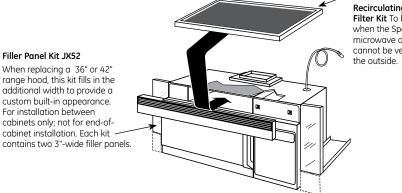
Filter Kit JX81H– Recirculating Charcoal Filter Kit To be used when the Spacemaker microwave oven cannot be vented to the outside
