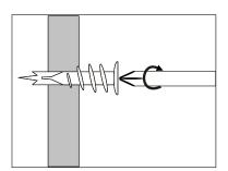
Note: Whenever possible, the hood should be secured to wood studs celling and/or wall with minimum thickness 3/8".
