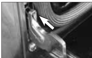
Fig. 25 Hinge retainer clip in locked position
