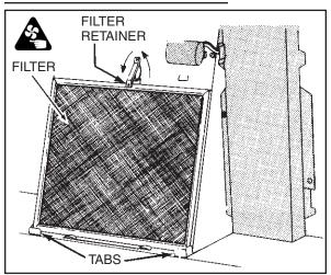
Remove aluminum filter by turning filter retainer to one side. Filter should be washed once a month in a hot detergent solution. Aluminum filters are dishwasher safe. When installing filter, make sure that filter slides under retaining tabs on back of fan housing. Turn filter retainer so that arrows on retainer point toward front and back of hood.
