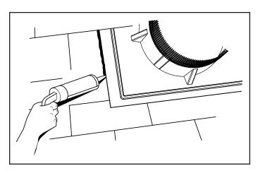
15. Using a good grade of roofing cement material, seal shingles and all nail heads. DO NOT seal the bottom edge of the ventilator base.
