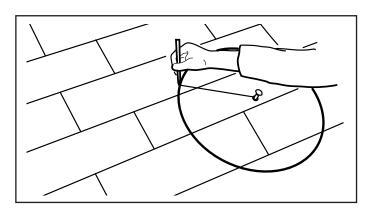
7. From the roof side, using the guide hole as the center point, use a nail and string to scribe a 16-1/2" diameter circle on the shingles. Note: If replacing an existing ventilator, the hole diameter may be larger than 16-1/2". This is acceptable provided the roofing material overlaps the ventilator by at least 1" on all sides.
