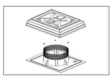
16. Install the ventilator dome to the ventilator base using the four (4) stainless steel 5/16" sheet metal screws removed during step 4.
