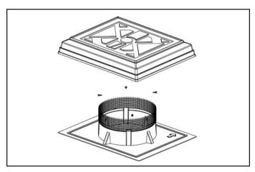
Separate the ventilator dome from the ventilator base by removing the four (4) stainless steel 5/16" sheet metal screws. Lift the ventilator dome off the ventilator base and proceed to the following steps.
