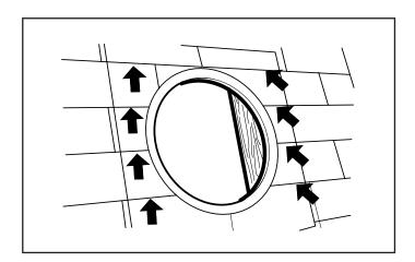
12. For proper removal of roofing nails, draw a 26" square, centered around the hole. Remove nails holding shingles down from top two-thirds of square.
