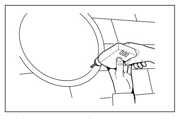
10. Drill a large starting hole for the sabre saw just inside of the line or the 14" circle created in Step 8.
