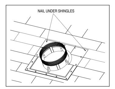
14. Make sure the ventilator base is parallel to the roof ridge, carefully lift shingles and nail or screw base securely to the roof using galvanized roofing nails or screws. Nail all corners and around perimeter of base every 6 inches.
