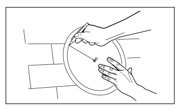
9. Using the same nail and string shown in step 6, scribe a 14" diameter circle on the black paper or roof decking. Note: if replacing an existing ventilator the hole diameter may be larger than 14". This is acceptable provided the ventilator base is adequately supported by the roof decking.
