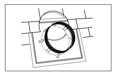
13. Apply a large bead of roofing cement in the molded groove on the bottom side of ventilator base. Making sure the arrow on the ventilator base is pointed toward the roof ridge, start two-thirds of the way down from the top of the 26" square and slide the ventilator base under the shingles. Do not bend the shingles any more than necessary. Center the ventilator base over the hole.
