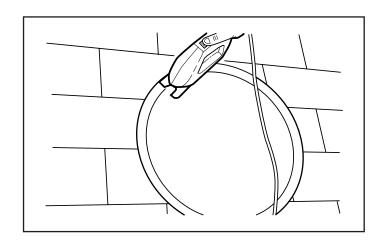
11. Cut out the roof board(s) inside of the line.
