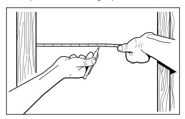
5. Working from the inside of your attic, find the desired ventilator location and mark a spot halfway between rafters at a point that is 24" – 36" below the roof ridge.
