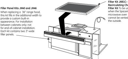
Recirculating Charcoal Filter Kit To be used when the Spacemaker microwave oven cannot be vented to the outside.
