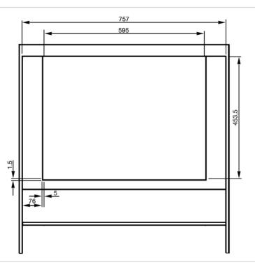
• Trim kit for SU45MCX to install in wider wall cabinets above a 30" oven. The kit consists of two stainless steel bars that allow the speed oven to reach 30" wide.
