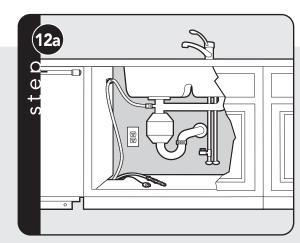
(Discharge with food waste disposer) **Note:** Be sure to remove the knockout or plug from the fitting of the disposer before connecting drain line.
