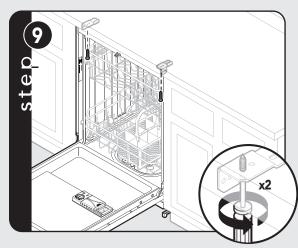
Attach screws through bracket into cabinets.
