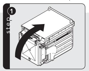
Remove any loose items in the dishwasher and carefully lay the dishwasher on its back. **Note:** Be careful not to
