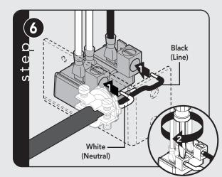
Connect wires to terminal block.
