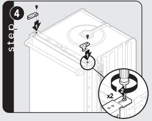
Attach brackets with two screws (1 per bracket).
