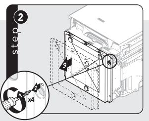
Remove bottom pan. **Note:** Rapid removal of the bottom pan will cause damage to the moisture sensor. For installation and servicing, slowly pull the bottom pan from the unit and disconnect the wire from the moisture sensor, which is located in the center of the pan.
