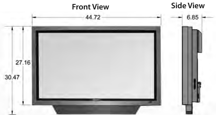
Dimensions with detachable speaker module. All measurements are in inches
