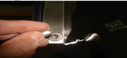
7) Turn the door over and remove the two screws that are on the left side. Save the screws for the next step.
