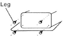
If the floor is uneven, adjust the legs. Do not insert pieces of wood or any other object under the legs.
