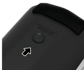
<The Smart Touch Control's pairing button>
