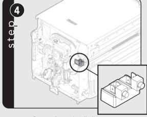
Remove factory installed power cable from terminal block.
