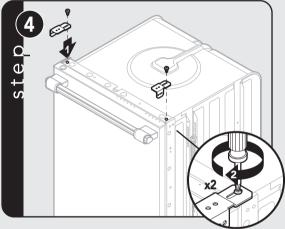
Attach brackets with two screws (1 per bracket).
