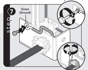
Connect ground wire. Tighten screws on strain relief.
