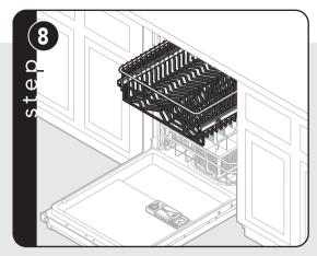
To check level, front to back, pull the top rack half-way out of unit. The rack should remain stationary and not move in or out. Note: Leveling is important for optimal performance.
