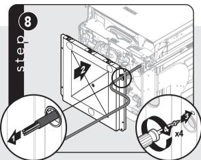
Run wire through grommet on bottom pan.
