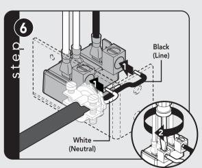
Connect wires to terminal block.
