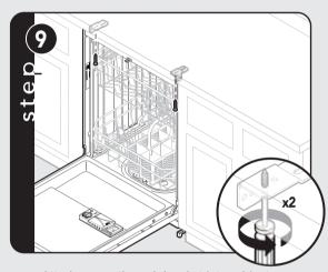
Attach screws through bracket into cabinets.
