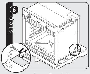
Unscrew pallet screws from side of oven.
