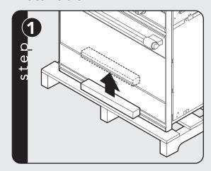
Remove wooden brace on front of pallet.
