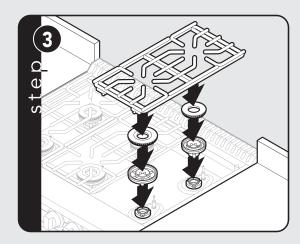
Burner caps are packed in cardboard top pack with the grates. Place burner on top of range. Place burner grate on top of burner cap and grate support.
