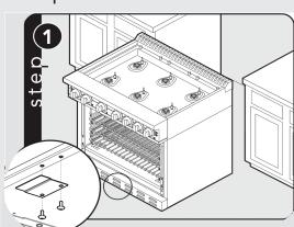
The kickplate bracket and scews (2) are located with the antitip bracket. Without removing the kickplate and using a short screw driver, install the bracket on the inside of the kickplate using the two screws provided.
