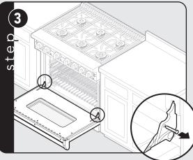
Remove pins from hole in hinges.
