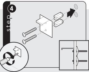
Attach bracket with mounting hardware provided.
