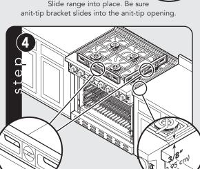
Check that unit is level side to side and front to back. The side trim must be 3/8" (0.95 cm) above countertop. If unit is not level repeat Steps 5-7 of "Leveling/Adjustments/Alignment" section.
