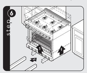
Lift unit and prop on wood blocks.
