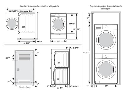
\* Required spacing \*\* External exhaust elbow requires additional space.
